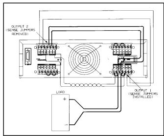
Figure 4-11. Parallel Connections with Local Sensing
